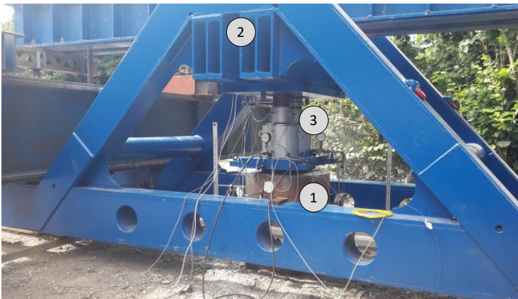
Figure 2: Hydraulic pressure unit for load tests fully assembled.
